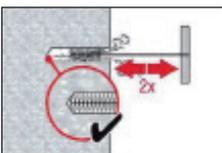
Brush 2 times with the specified brush size by inserting the steel brush Hilti HIT-RB to the back of the hole (if needed with extension) in a twisting motion and removing it.
