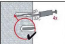
Blow out again with manual pump at least 4 times until return air stream is free of noticeable dust.
