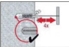
Brush 4 times with the specified brush size (brush  $\phi \geq \text{bore hole } \phi$ ) by inserting the steel brush Hilti HIT-RB to the back of the hole (if needed with extension) in a twisting motion and removing it.
