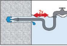
Flush 2 times the hole by inserting a water hose (water-line pressure) to the back of the hole until water runs clear.
