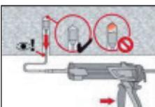
Overhead installation and/or installation with embedment depth  $h_{ef} > 250\text{mm}$ . For overhead installation the injection is only possible with the aid of extensions and piston plugs. Assemble HIT-RE-M mixer, extension(s) and appropriately sized piston plug HIT-SZ. Insert piston plug to back of the hole and inject adhesive. During injection the piston plug will be naturally extruded out of the bore hole by the adhesive pressure.
