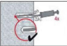
The Hilti manual pump may be used for blowing out bore holes up to diameters  $d_0 \leq 20\text{ mm}$  and embedment depths up to  $h_{ef} \leq 10d$ .
