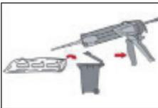
The foil pack opens automatically as dispensing is initiated. Discard initial adhesive. Depending on the size of the foil pack an initial amount of adhesive has to be discarded.
