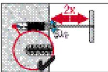
Brush 2 times with the specified brush size (brush  $\phi \geq$  bore hole  $\phi$ ) by inserting the steel brush Hilti HIT-RB to the back of the hole (if needed with extension) in a twisting motion and removing it.
