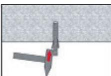
For overhead installation use piston plugs and fix embedded parts with e.g. wedges HIT-OHW
