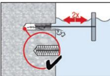
Brush 2 times with the specified brush size (brush  $\varnothing \geq$  bore hole  $\varnothing$ ) by inserting the steel brush Hilti HIT-RB to the back of the hole (if needed with extension) in a twisting motion and removing it.
