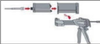
Tightly attach new Hilti mixing nozzle HIT-RE-M to foil pack manifold (snug fit). Do not modify the mixing nozzle. Observe the instruction for use of the dispenser. Check foil pack holder for proper function. Do not use damaged foil packs / holders. Swing foil pack holder with foil pack into HIT dispenser.
