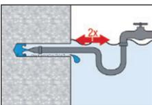
Flush the hole again 2 times by inserting a water hose (water-line pressure) to the back of the hole until water runs clear.
