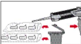
The foil pack opens automatically as dispensing is initiated. Discard initial adhesive. Depending on the size of the foil pack an initial amount of adhesive has to be discarded.
