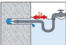
Flush the hole again 2 times by inserting a water hose (water-line pressure) to the back of the hole until water runs clear.
