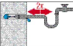
Flush 2 times the hole by inserting a water hose (water-line pressure) to the back of the hole until water runs clear.
