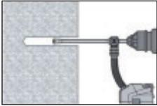
Drill hole to the required embedment depth with an appropriately sized Hilti TE-CD or TE-YD hollow drill bit with Hilti vacuum attachment. This drilling system removes the dust and cleans the bore hole while drilling when used in accordance with the user's manual.
