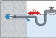
Flush 2 times the hole by inserting a water hose (water-line pressure) to the back of the hole until water runs clear.
