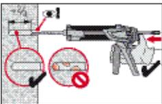
Inject the adhesive starting at the back of the hole, slowly withdrawing the mixer with each trigger pull. Fill holes approximately 2/3 full. It is required that the annular gap between the anchor and the concrete is completely filled with adhesive along the embedment length.
