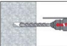
Drill Hole to the required embedment depth with a hammer drill set in rotation-hammer mode using an appropriately sized carbide drill bit.
