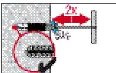
Brush 2 times with the specified brush size (brush  $\varnothing \geq$  bore hole  $\varnothing$ ) by inserting the steel brush Hilti HIT-RB to the back of the hole (if needed with extension) in a twisting motion and removing it.
