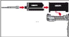
Tightly attach new Hilti mixing nozzle HIT-RE-M to foil pack manifold (snug fit). Do not modify the mixing nozzle. Observe the instruction for use of the dispenser. Check foil pack holder for proper function. Do not use damaged foil packs / holders. Swing foil pack holder with foil pack into HIT dispenser.
