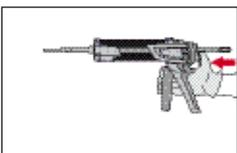
After injection is completed, depressurise the dispenser by pressing the release trigger. This will prevent further adhesive discharge from the mixer.
