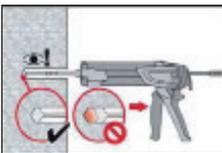
Inject the adhesive starting at the back of the hole, slowly withdrawing the mixer with each trigger pull. Fill holes approximately 2/3 full. It is required that the annular gap between the anchor and the concrete is completely filled with adhesive along the embedment length.
