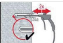
Blow 2 times from the back of the hole (if needed with nozzle extension) over the hole length with oil-free compressed air (min. 6 bar at 6 m<sup>3</sup>/h) until return air stream is free of noticeable dust. Bore hole diameter  $\geq 32\text{ mm}$  the compressor must supply a minimum air flow of 140 m<sup>3</sup>/hour.
