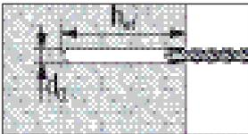
Drill Hole to the required embedment depth with a hammer drill set in rotation-hammer mode using an appropriately sized carbide drill bit.
