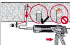
Overhead installation and/or installation with embedment depth  $h_{ef} > 250\text{mm}$ . For overhead installation the injection is only possible with the aid of extensions and piston plugs. Assemble HIT-RE-M mixer, extension(s) and appropriately sized piston plug HIT-SZ. Insert piston plug to back of the hole and inject adhesive. During injection the piston plug will be naturally extruded out of the bore hole by the adhesive pressure.
