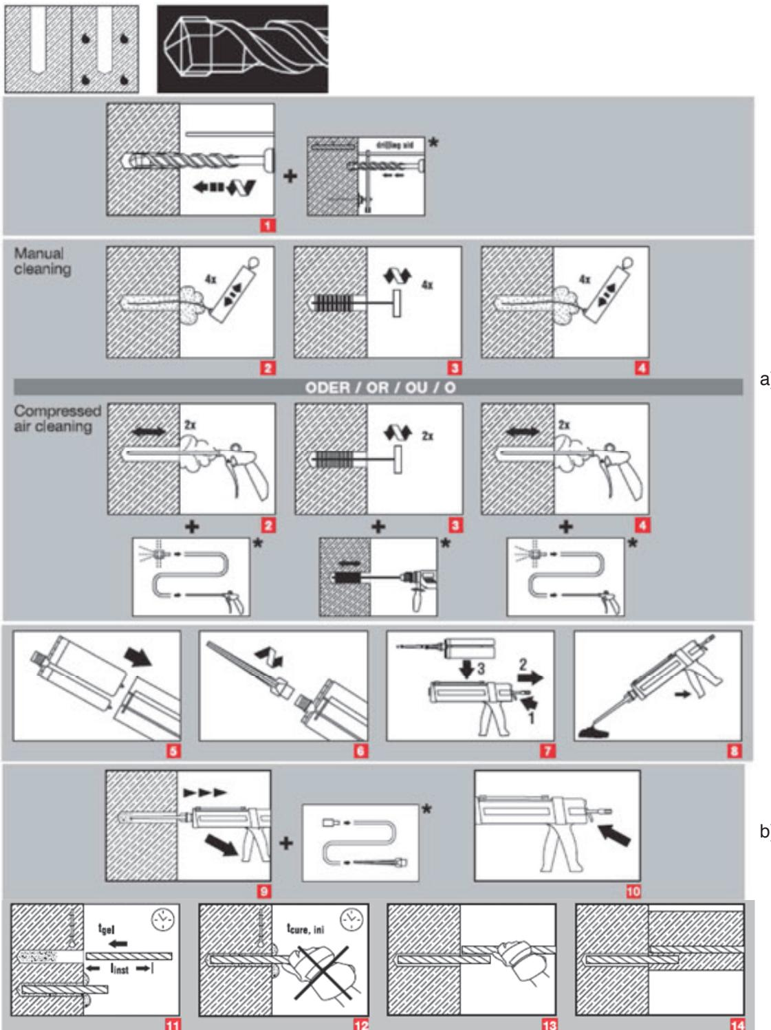
**a)** Note: Manual cleaning for drill hole sizes  $d_0 \leq 18\text{mm}$  and embedment depth  $h_{ef} \leq 10\text{ d}$  only!
