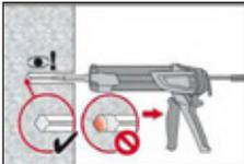
Inject the adhesive starting at the back of the hole, slowly withdrawing the mixer with each trigger pull. Fill holes approximately 2/3 full. It is required that the annular gap between the anchor and the concrete is completely filled with adhesive along the embedment length.
