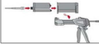
Tightly attach new Hilti mixing nozzle HIT-M1 to foil pack manifold (snug fit). Do not modify the mixing nozzle. Observe the instruction for use of the dispenser and the mortar. Check foil pack holder for proper function. Do not use damaged foil packs / holders. Insert foil pack into foil pack holder and put holder into HIT dispenser.
