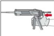
After injection is completed, depressurise the dispenser by pressing the release trigger. This will prevent further adhesive discharge from the mixer.
