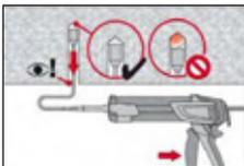
Overhead installation and/or installation with embedment depth  $h_{ef} > 250\text{mm}$ . For overhead installation the injection is only possible with the aid of extensions and piston plugs. Assemble HIT-M1 mixer, extension(s) and appropriately sized piston plug HIT-SZ. Insert piston plug to back of the hole and inject adhesive. During injection the piston plug will be naturally extruded out of the bore hole by the adhesive pressure.
