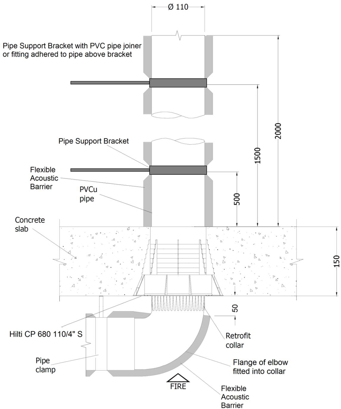
**Figure 4 – uPVC pipes flange of elbow fitted into firestop collar protected with Hilti CP 680 110/4" S + CP 680 N-RAD Cast-In Firestop Collar System without Ultrafloor, optional flexible acoustic barrier at least 50mm from underside of concrete slab**
