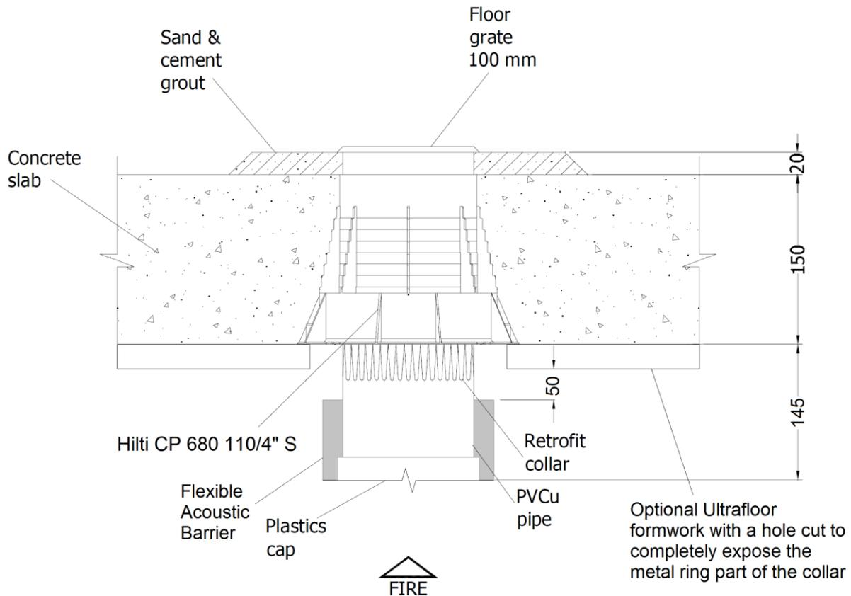
**Figure 1** – uPVC floor waste – straight pipe protected with CP 680 110/4" S + CP 680 N-RAD Cast-In Firestop Collar System with Ultrafloor, optional flexible acoustic barrier at least 50mm from underside of Ultrafloor
