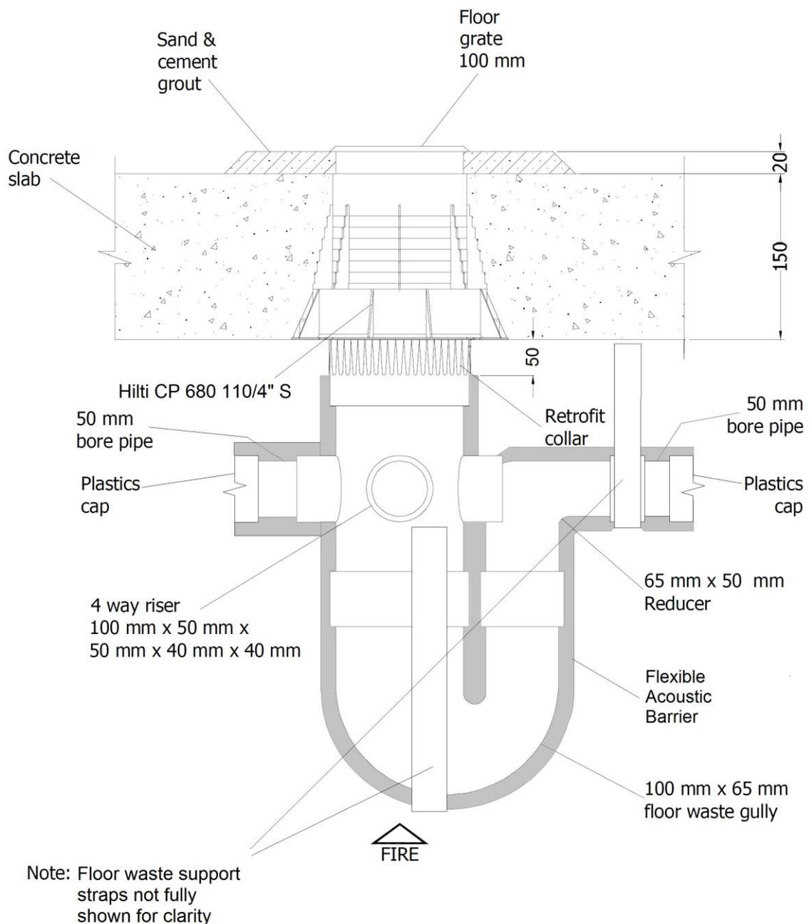
**Figure 8** – uPVC floor waste – gully pipe protected with Hilti CP 680 110/4\" S and Hilti CP 680 110/4\" N-RAD without Ultrafloor, optional flexible acoustic barrier at least 50mm from underside of concrete slab
