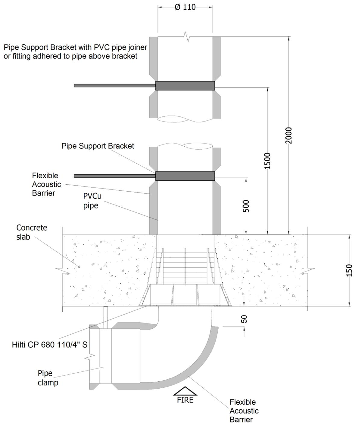
**Figure 6 – uPVC pipes flange of elbow fitted outside firestop collar protected with Hilti CP 680 110/4" S Cast-In Firestop Collar without Ultrafloor, optional flexible acoustic barrier at least 50mm from underside of concrete slab**
