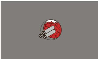
**Pack mineral wool.** Leave sufficient depth for applying Hilti Firestop Intumescent Sealant CP 611A..
