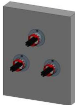
Zero distance (horizontal/vertical distance between flanges linear or cluster)
