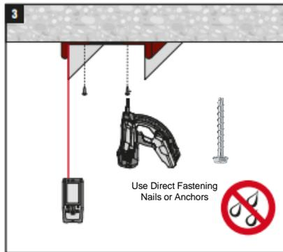
Fasten the top track with the CFS-TTS to the underside of the slab. Ensure surfaces are clean and dry.
