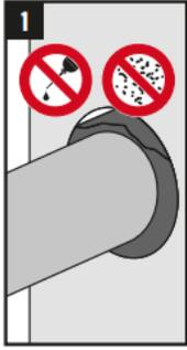
1 Ensure that the surface and the pipe are clean and that the Hilti CP 606 seal in the annular gap has cured.
